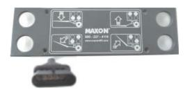
Test of the sensor-switch in the platform:platform closed and lift on:LED lights.Power supply Ok.platform position0 ° till ca. 60 °:LED outSensor-switch S1 is Ok.
