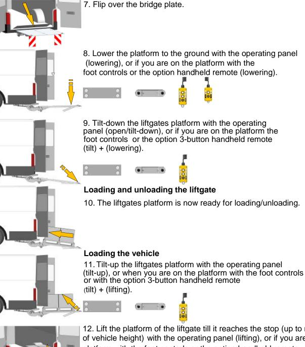
12. Lift the platform of the liftgate till it reaches the stop (up to marking of vehicle height) with the operating panel (lifting), or if you are on the platform with the foot controls or the option handheld remote (lifting).
