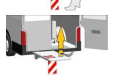
18. Lift the platform of the liftgate up till stop with the operators panel (lifting), or if you are on the platform with the foot controls or the option handheld remote (lifting).
