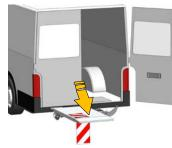
3. Open the platform with the operating panel (open/tilt-down) or on the option 3-button handheld (tilt) + (lowering).
