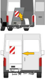
19. Close the platform with the operating panel (tilt-up) or the option 3-button handheld remote (tilt) + (lifting).
