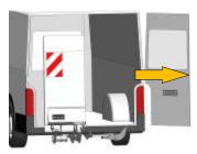
2. Open the right rear door to get access to the operating panel or to the option 3-button handheld cabled remote.
