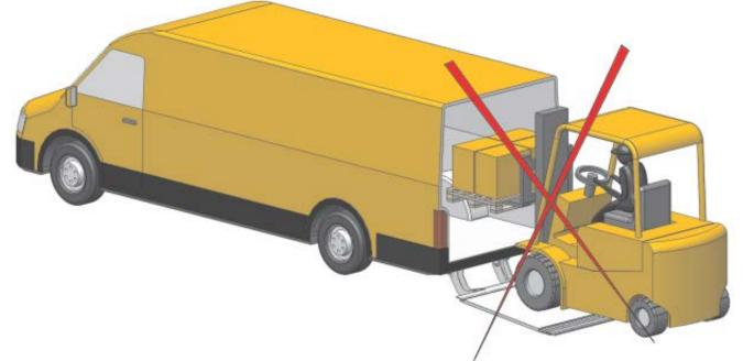
By any loading or unloading the vehicle must be secured, so it does not roll away. (Activate parking brake).
