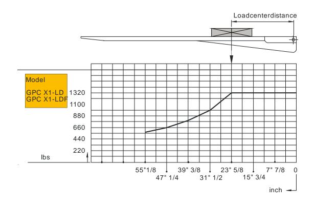
The maximum loading capacity specified in the loading diagram must not be exceeded. The platform may not be used as a bridge plate.
